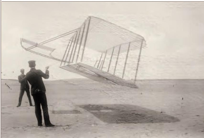
The photograph above shows the Wright Brothers at Kitty Hawk, North Carolina, with their 1901 Glider being flown as a kite. It weighed 98 pounds and had a wingspan of 22 feet. The kite appears to be floating in the air, but it is actually being held motionless because the forces that are acting on it are “balanced.”
